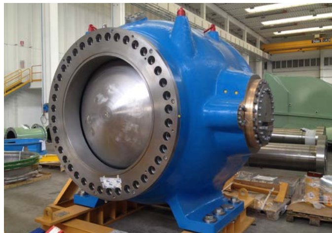
Valve in manufacturing, Grand Maison, Romanche Valley
