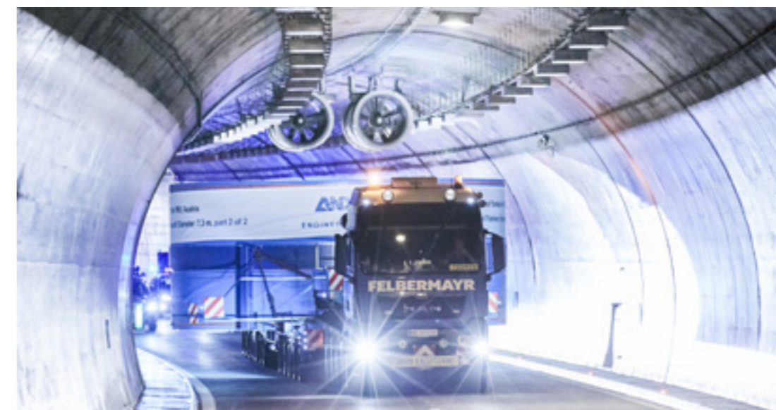
Based on the unique ANDRITZ engineering and logistics concept, the Yankee was transported in two halves and assembled on site.
