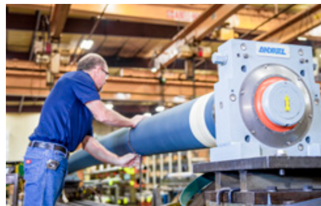
Completed spreader roll in high-speed quality control station
