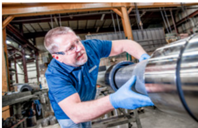
All metal spreader roll during spool assembly
