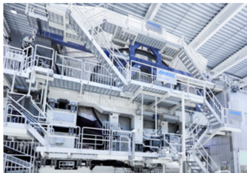
The 24 ft MG steel Yankee is the largest of its kind worldwide.
