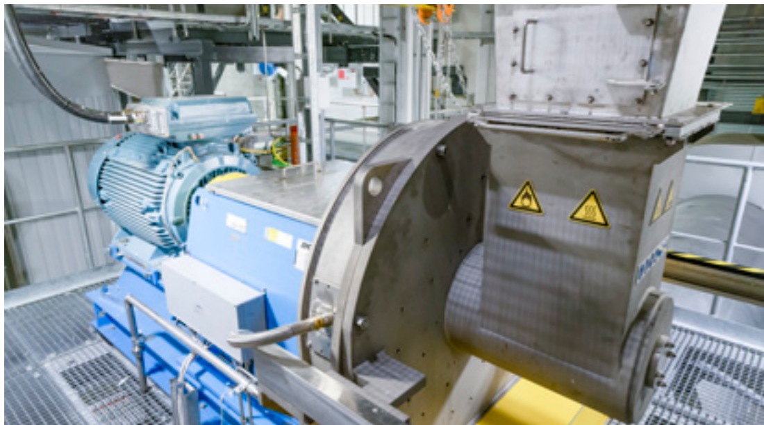
The HC-Fluffer breaks up fiber particles. The fluffed pulp is well-prepared for the further drying process.
