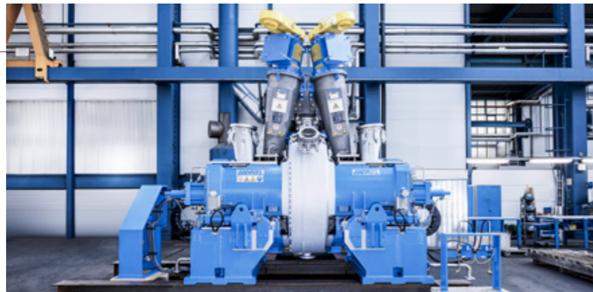
ANDRITZ TX68 refiner with DoubleSEPF (Side Entry Plug Feeder) and C-Feeder (Constant Feeder)
