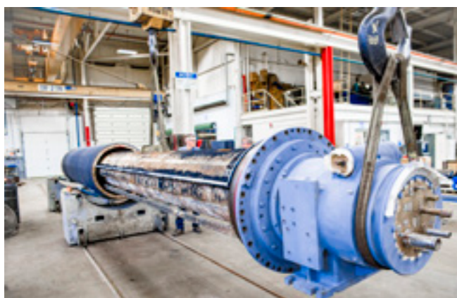
Suction box being removed from suction roll
