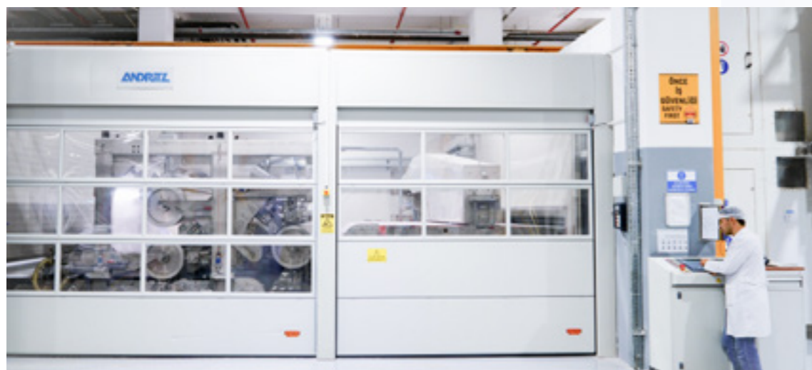
JetlaceEssentiel hydroentanglement unit with neXjet injector state-of-the-art
