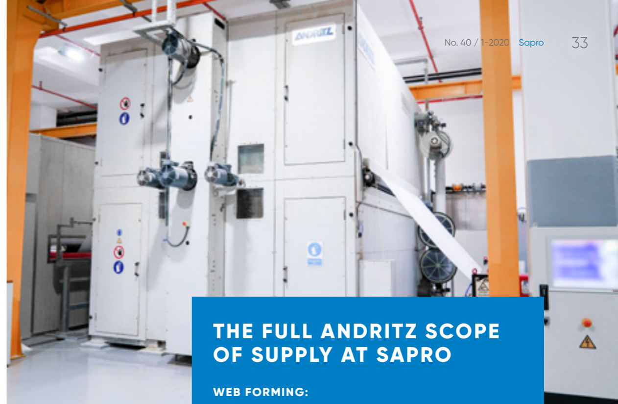
neXdry dryer with heat recovery
