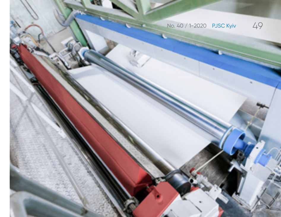
The new PrimeCal Hard hard-nip calender from ANDRITZ achieved the agreed smoothness parameters soon after start-up.
