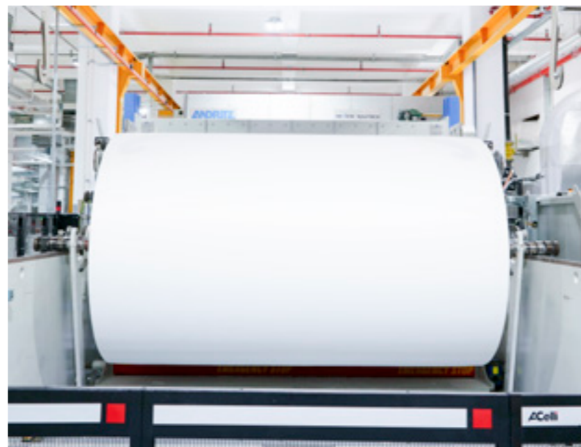
End of line: Jumbo ready to be used in the converting line
