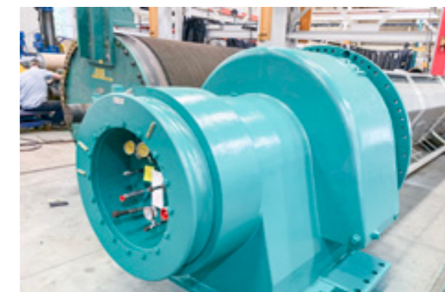
Refurbished suction box
