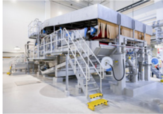
The ANDRITZ Twin Wire Press has been proven in many applications for all pulp types and is the best suited thickening equipment prior to a Flash Dryer.
