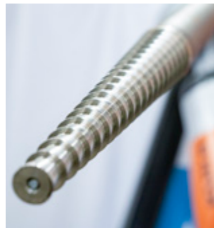
On the end of the arm is a specially designed tool that cleans away the solidified smelt.
