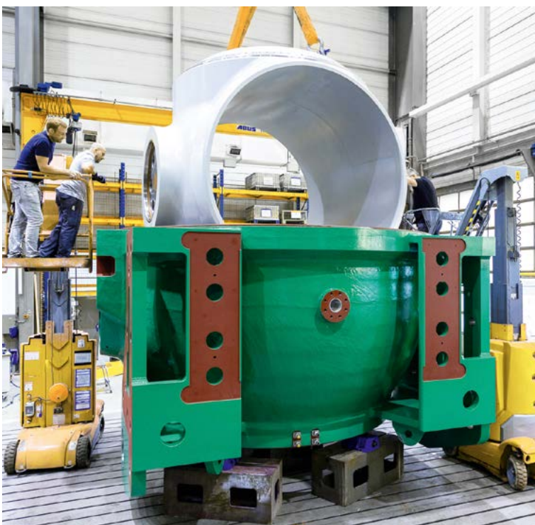
Assembly of valve rotor into MIV housing
