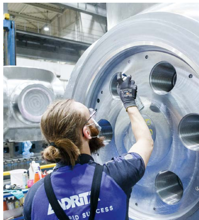
Crack inspection on sealing surfaces of the valve rotor
