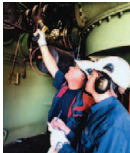
Juha Welling (left), ASIP's Fiberline specialist, checks the heat profile of operating equipment with a non-contacting temperature gauge. Recording the results is Lauri Welling.
