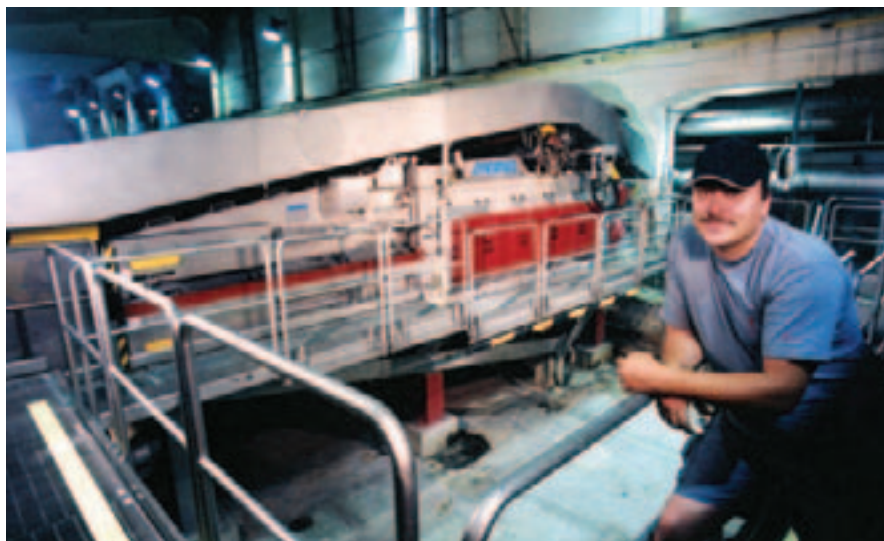
Bleach plant Superintendent, Göran Larsson, near one of two new Andritz Twin Wire presses (3.6 m working width) in the post-bleach wash position.
