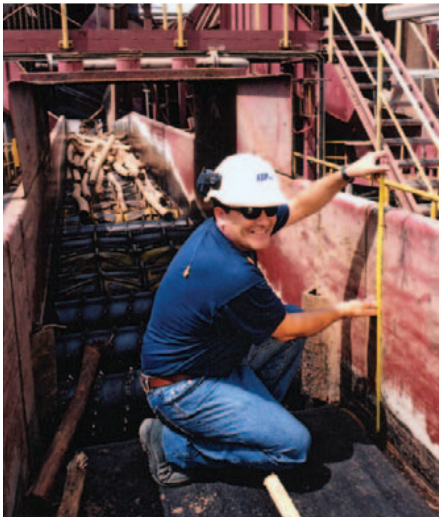
José Eduardo takes measurements in the field to design a modification to the log delivery system in the woodyard at Setubal.
